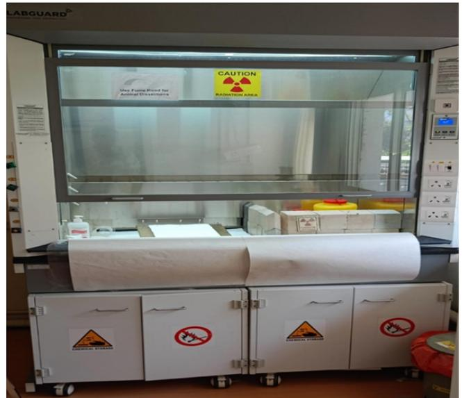
Fig.7: Fume-hood facility: Employed for handling radioactivity for animal experiments.
