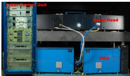
Typical Copper Vapor Laser with High voltage pulse power supply
